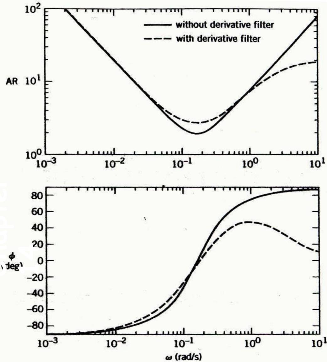
Figure Bode plots of ideal parallel PID controller and series PID controller with derivative filter ( $\alpha = 1$ ).
